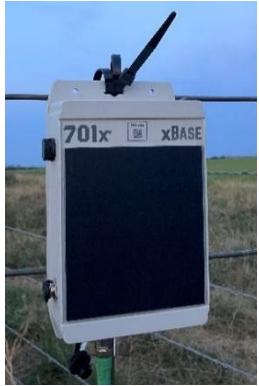
The XBASE system, 701x, uses a pressure transducer in the tank to sense the depth of water above the sensor as well as the temperature of the water. The system proposes to update the website about every 2 hours (cellular communication). In addition, the system proposes to send a notification to one or more cell phones when the water in the tank drops below an alert level the producer specified or if the temperature of the water becomes greater than a specified temperature.
